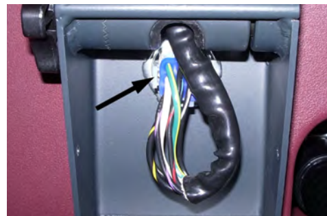
7. The wire harness must be aligned with the patterns on the connector to fit.
