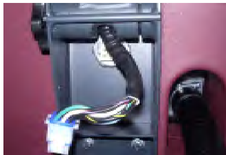
6. Attach the wire harness to the machine.
